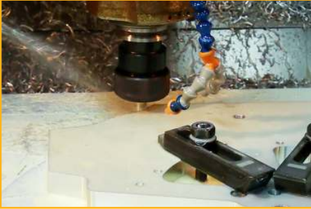
GEO-119C Using VoluMill with CAMWorks, Tomak is able to develop fixtures to hold aircraft engine parts for fast hole EDM
