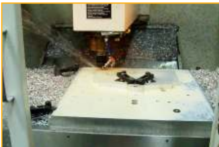
GEO-119B Tomak processes an aircraft engine parts fixture on its Fadal VMC 6030
