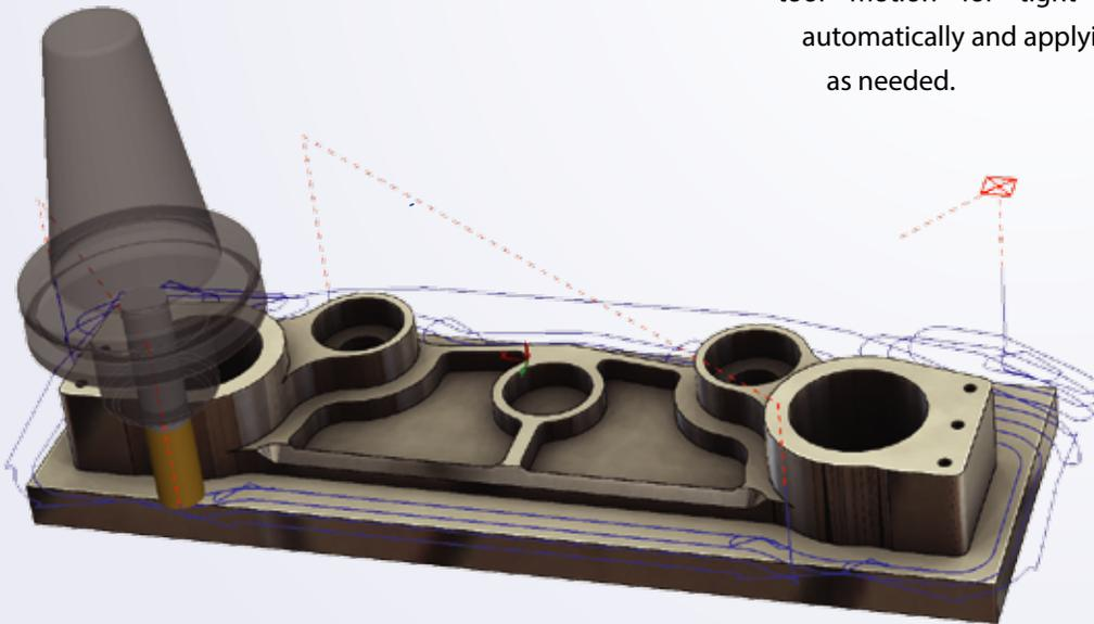
milling for any type of geometry is created quickly and easily. The toolpaths are created for constant motion, thus reducing cycle time and extending cutting-tool life by reducing stress on machine tools.
