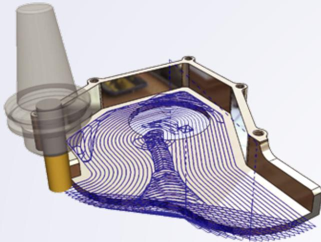
VoluMill's unique approach to high speed material removal assists the programmer to determine the optimum material removal rate for any combination of part geometry, material, machine, and cutting tool. Material is removed in the most effective way possible. Consequently, machines run smoothly and tools run cooler.
